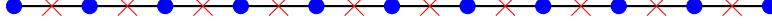
FIGURE 1. The red crosses stand for the centered grid while the blue dots are for the staggered grid
